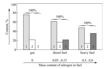
Fig. 2. Nomogram of the distribution of types of NOX for different types of fuel 1 - thermal; 2 - fast; 3 - fuel
