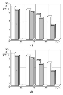
**Fig. 4.** Dependence of  $NO_X$  emission of ship diesel 6L20 Wartsila on  $N_e$  load for different degrees of opening of the gas bypass valve  $\Delta_{wg}$ :
