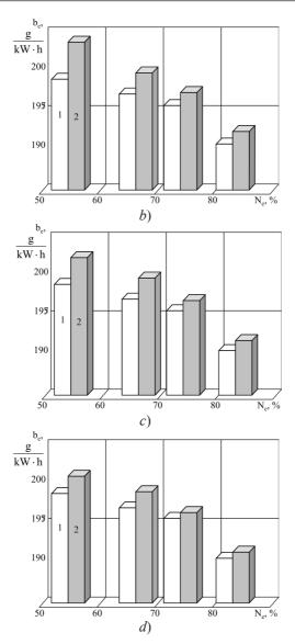
Fig. 5. The dependence of the specific effective fuel consumption be of a 6L20 Wartsila diesel engine on the Ne load for different degrees of opening of the gas bypass valve  $\Delta_{wg}$ :
